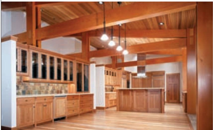
more contemporary structures use the metal connections as design elements that are connected by wood members.
